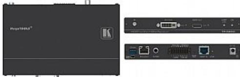
TP-588D is a high-performance, extended-reach HDBaseT 1.0 receiver for 4K60Hz (4:2:0) DVI or HDMI, Ethernet, RS-232, IR and stereo audio signals over twisted pair. It extends video signals to up to 100m (330ft) over CAT copper cables at up to 4K@60Hz (4:2:0) 24bpp video resolution and provides even further reach for lower HD video resolutions
